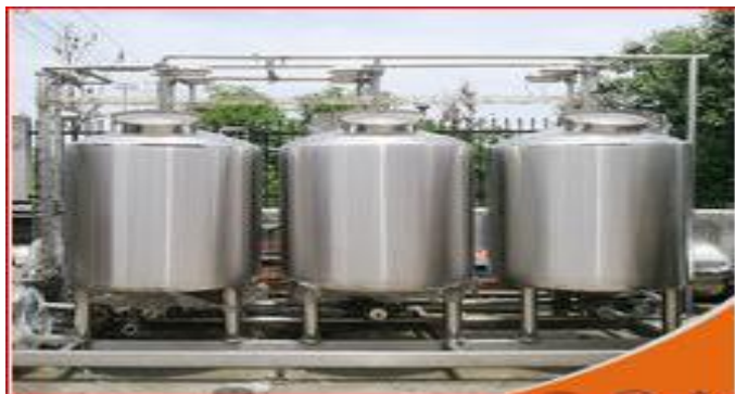
Figure 11 Clean in place /CIP/
